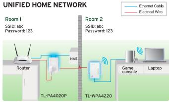
\*The powerline adapters need to be connected in the same electrical circuit.
