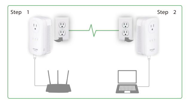
Note: Powerline adapters should be deployed on the same circuit and in set of two or more. The first, connected to the router and others located elsewhere to enable connectivity in those locations.
