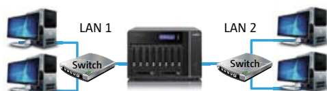
Support access of multiple IP from different LAN areas
